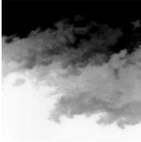
FIGURE 4. Example of a high-resolution image of the scalar field in a large-Reynolds-number separated shear layer recorded with laser-induced fluorescence.
